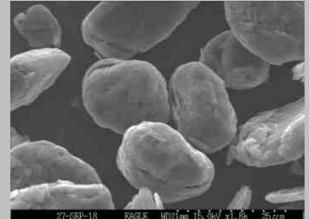
Battery spheroids – Goes into a lithium-ion battery
